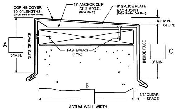
NOTE: Concealed splice plates must be field caulked to prevent water entry.
