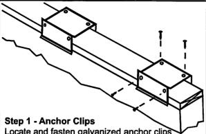
Locate and fasten galvanized anchor clips to wall at 2'6" centers with appropriate fasteners for substrate.
