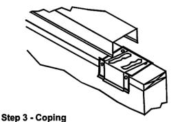
Install coping by pushing coping down until it engages. Field crimp inside face of the coping drip at each anchor clip, 2'6" O.C.
